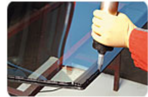
Elastic sealants used in bonding a car windshield.
