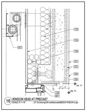
Compartmentalizing the Rain Screen Joinery; Strategic placement of weep tubes and or vents from floor line to floor line in multi-story buildings can prevent intruding water from running aimlessly through the building envelope before it is discovered at some distance from its entry.
