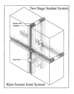
outside face of the wall, and seal against air and vapor passage on the interior side of the air space, where the *primary seal* is exposed to little of the destructive elements of weather and sun.
